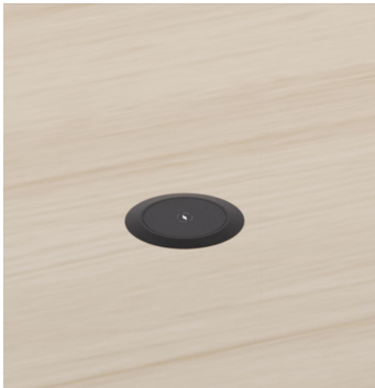
Multicharger Pro - AC085 Ø80mm support / Ø71mm cut out. Wireless charging + USB A
