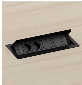
Electrification Box - AC056 319x154mm support / 294x147mm cut out. Surface electrical unit with 45° opening, metal box with folding top and 4 useful modules. Kit: 2 schukos points + 1 HDMI + RJ45 + cable connection strap 3 meters. White or black colour.
