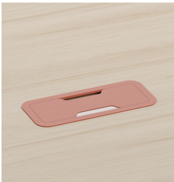
Top Access Rectangular - AC097 300x135mm support / 275x110mm cut out / 253x88mm passage. Rectangular metal top access with removable cover and double outlet. Customisable colour.
