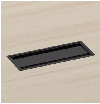
Top Access Double - AC062 320x135mm support / 313x128mm cut out. Top access double opening in metal. White or black colour.
